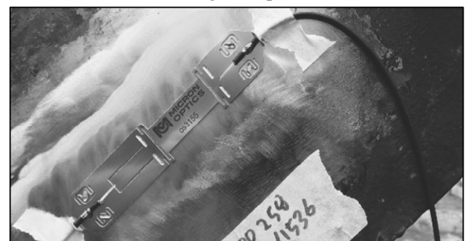
Figure 4 DFOS sensor mounted at the bottom chord of the old steel bridge and the FBG sensor SG7 is mounted very close to it at 14m from Abutment A, in order to
