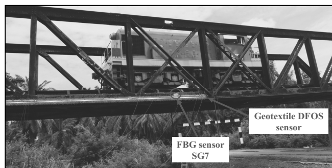
Figure 5 Installation of sensors
